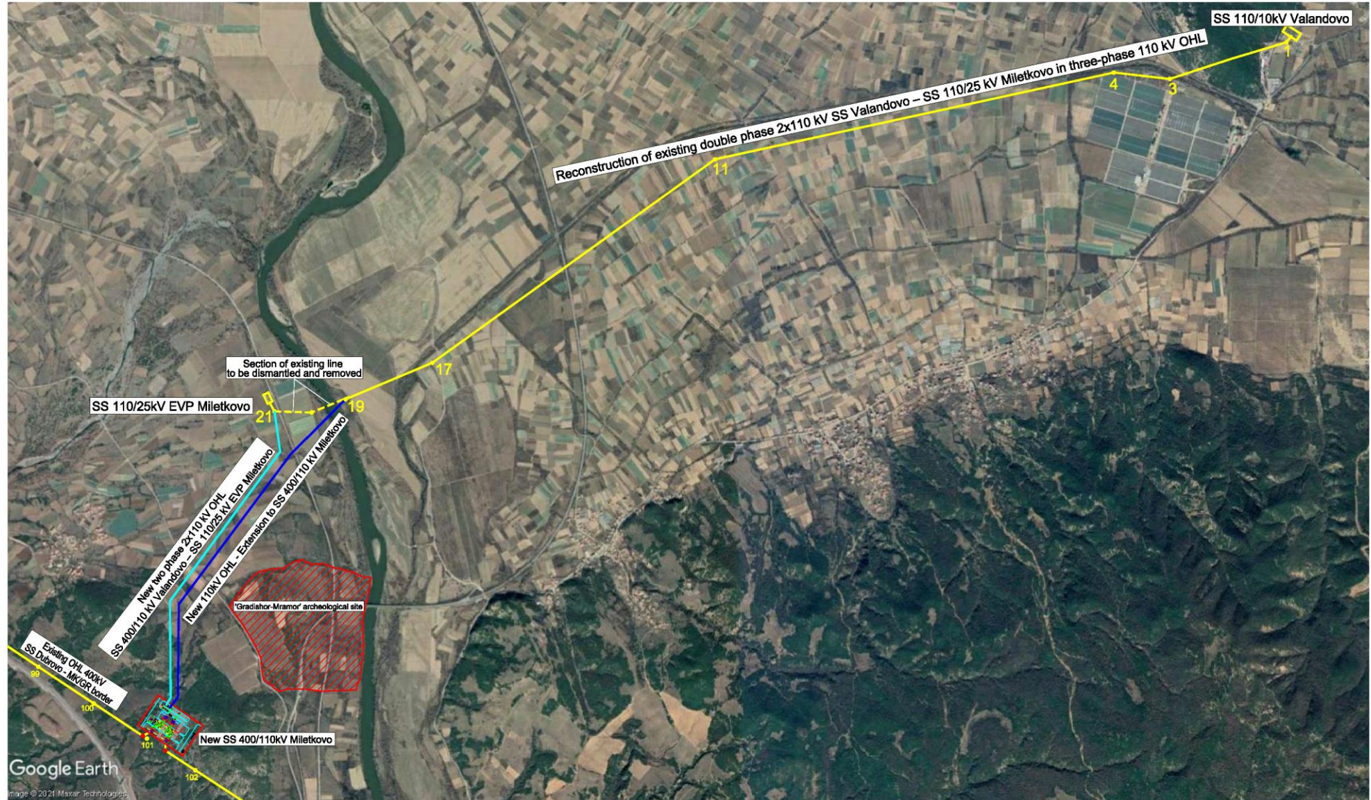
Figure 3.3: Reconstruction of existing transmission line from Valandovo substation to 'EVP' Miletkovo substation and extension to the new substation Miletkovo
